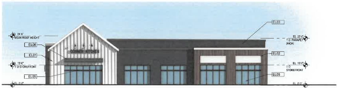
41 NORTH ELEVATION - SOUTH RETAIL - PHASE II SCALE 3/32" = 1'-0"
