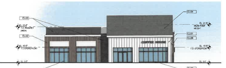
30 SOUTH ELEVATION - NORTH RETAIL - PHASE I SCALE 3/32" = 1'-0"
