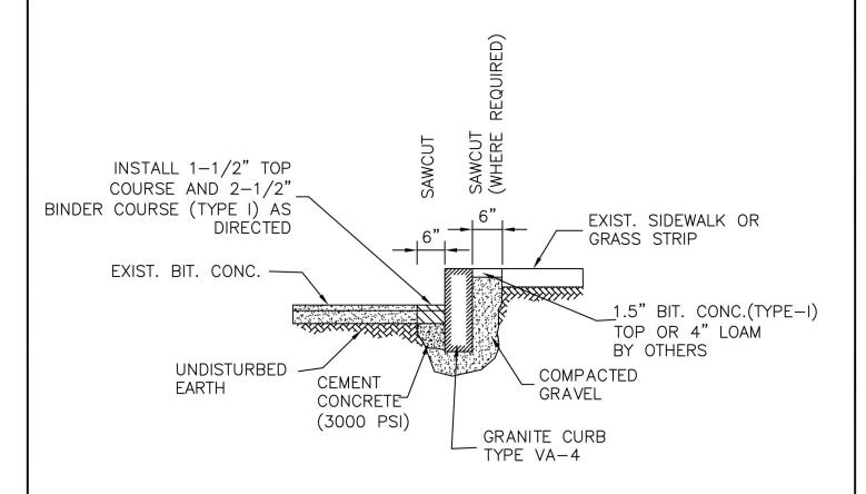
PER FOOT PRICE INCLUDES PAYMENT FOR SAWCUT, EXCAVATION, INSTALLATION OF GRANITE CURBING, CEMENT CONCRETE, GRAVEL, AND ANY INCIDENTAL WORK AS REQUIRED.
