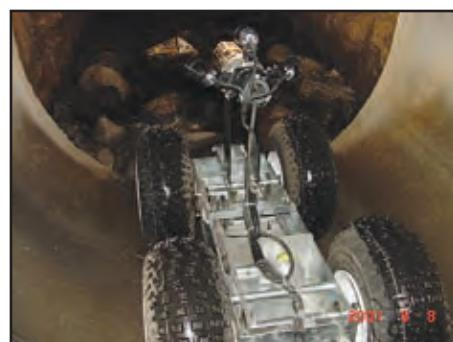
Figure 66: Tractor-mounted camera
