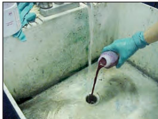
**Figure 63: Dye Testing Plumbing (NEIWPCC, 2003)****Dye Testing**
