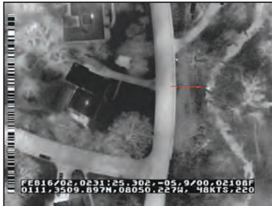
**Figure 72: Aerial thermography showing sewage leak**
