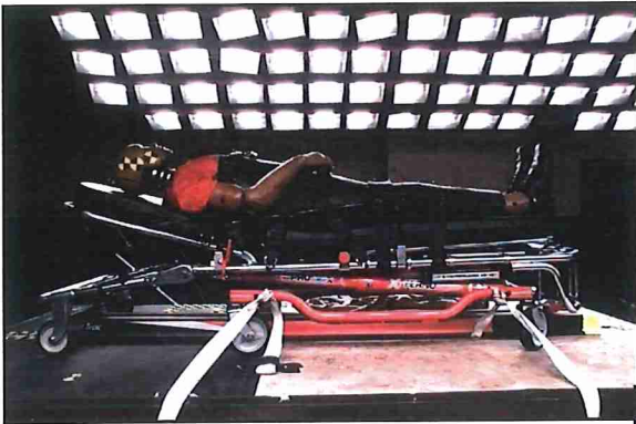
Production litter with new patient restraint and floor mount system
